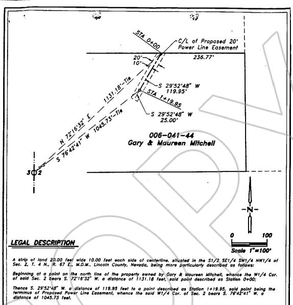
including a Guy Wire Easement extending S. 28'52'48" W. from Station 1+19.95 a distance of 25.00 feet.
