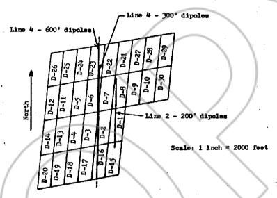
The survey was executed using frequency domain equipment operating at 2.5 Hs and 3 Hz. Line 2 was completed with 200 foot dipole spacings and read to N=5. Line 4 was completed using 300 foot dipole spacings and then expanded to 600 foot dipole spacings. Both spreads on Line 4 were read to N=5.
